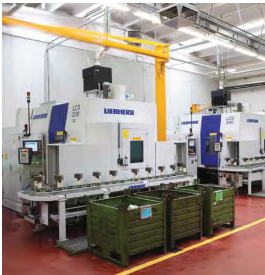
Versatile: the generating- and profile-grinding machine LCS 300
